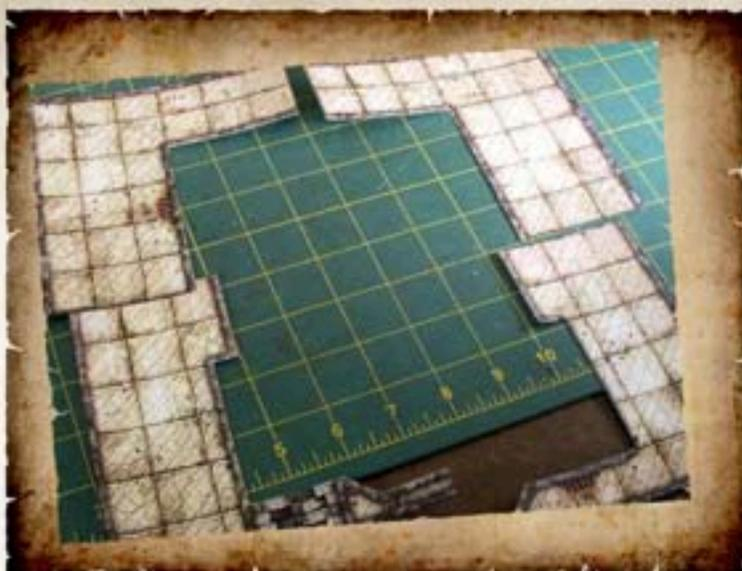
The tiles are already shaped to match the ground floor profile of the shop, so cut all four tiles out (test-fit them to be sure they're a good, tight fit and that you know where each one goes).
